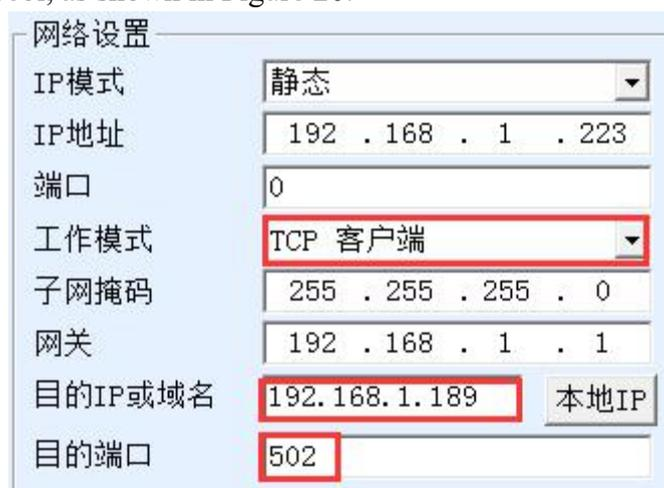
Figure 20 Modbus TCP Being client
