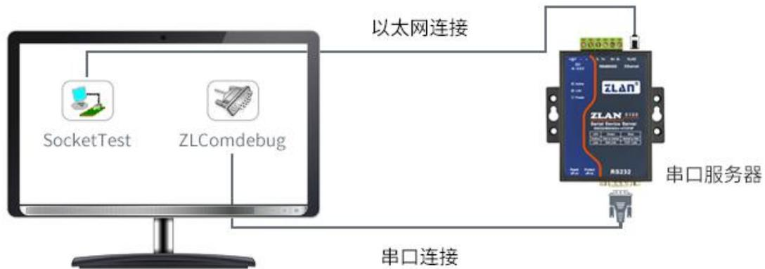
Figure 12 TCP Communication diagram
