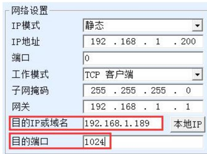
Figure 24The first destination IP address and port
