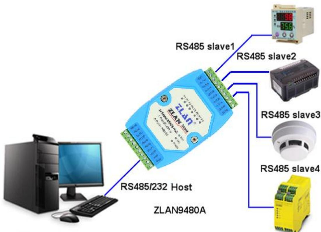
**Figure 2 ZLAN9480A connection diagram**
