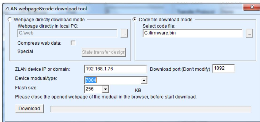
**Figure 35 ZLAN7104 Firmware Upgrade Method**
