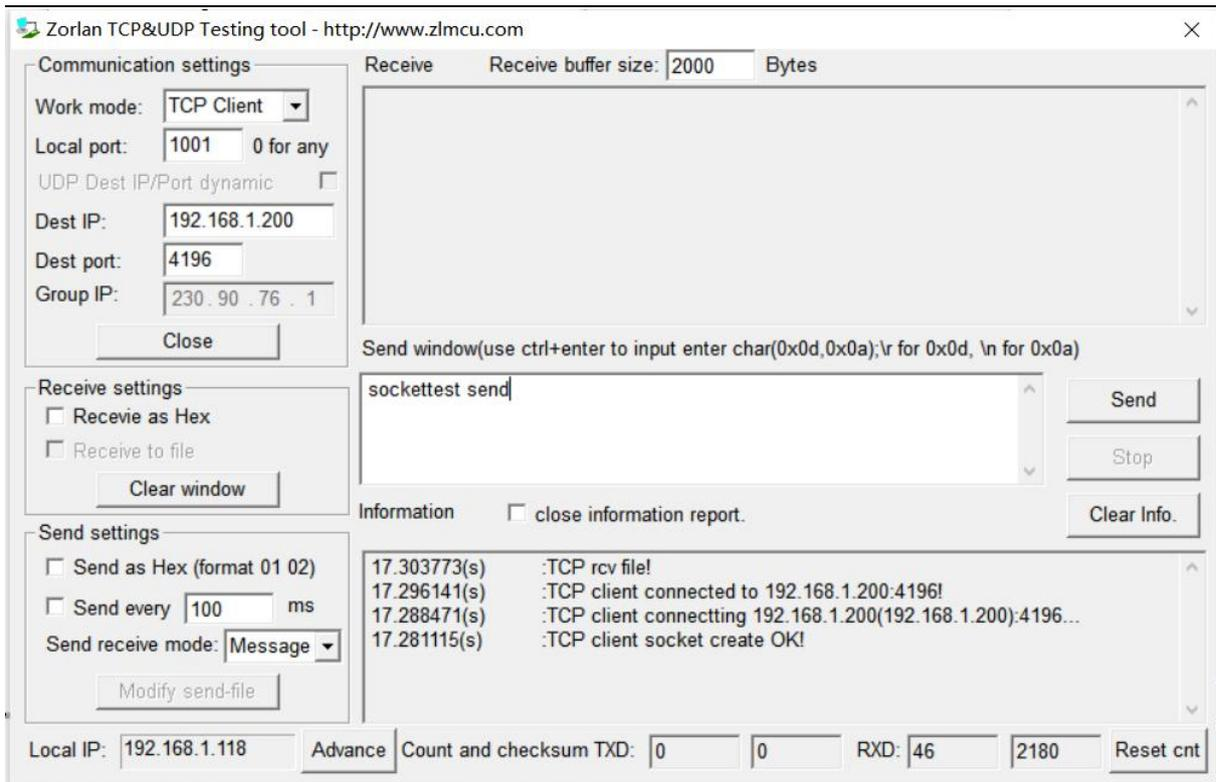
Figure 19 sockettest send and receive interface
