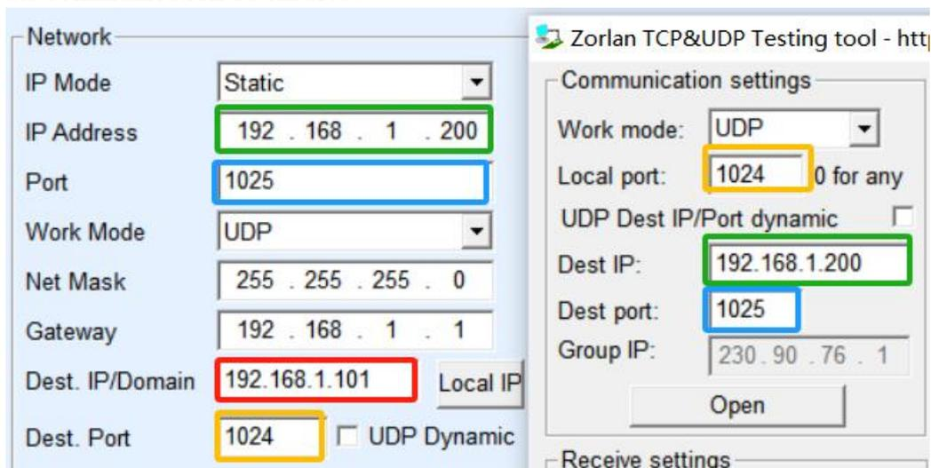
Figure 33 UDP Mode Parameter Configuration
