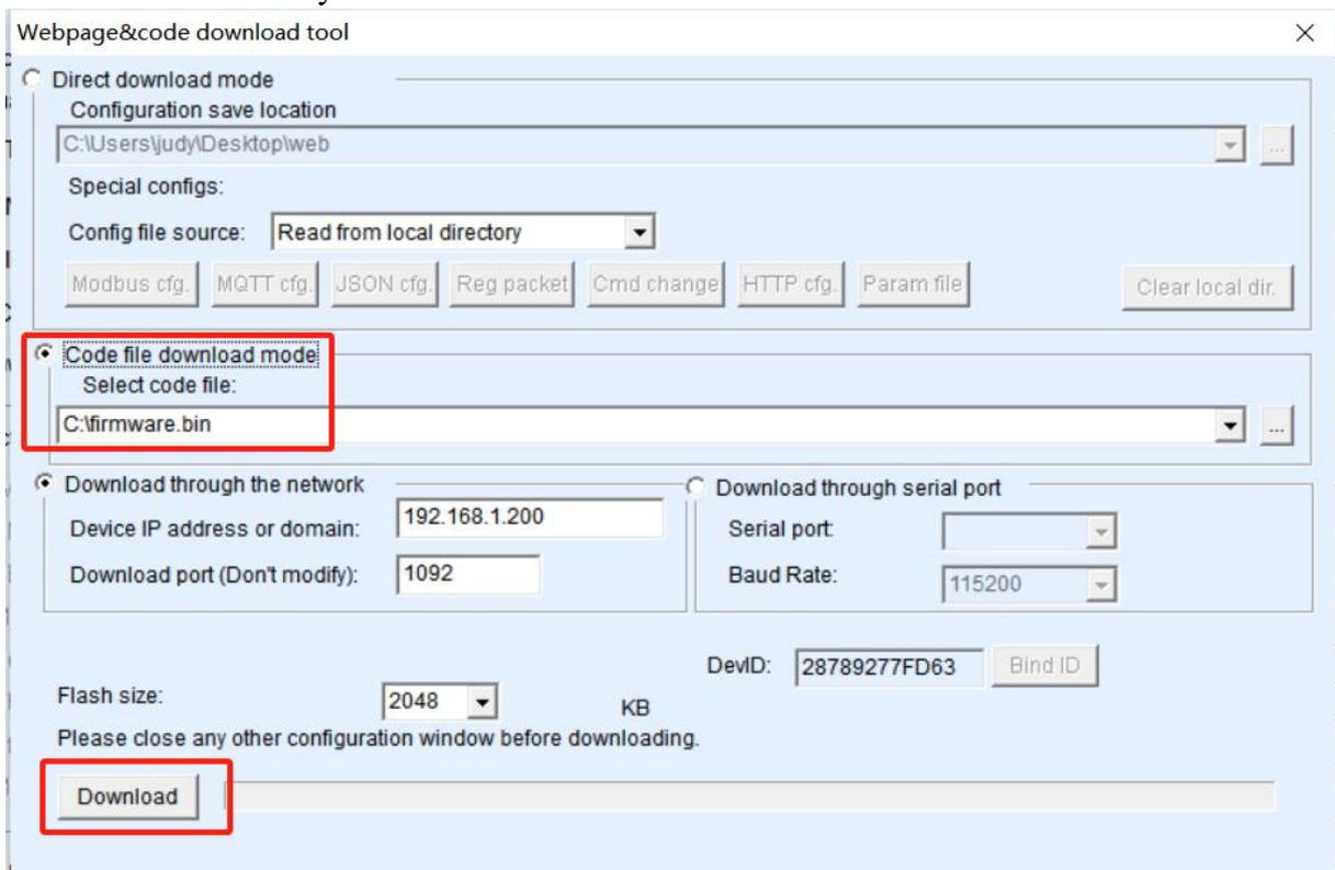
Figure 60 ZLAN7104M Firmware Upgrade Method
