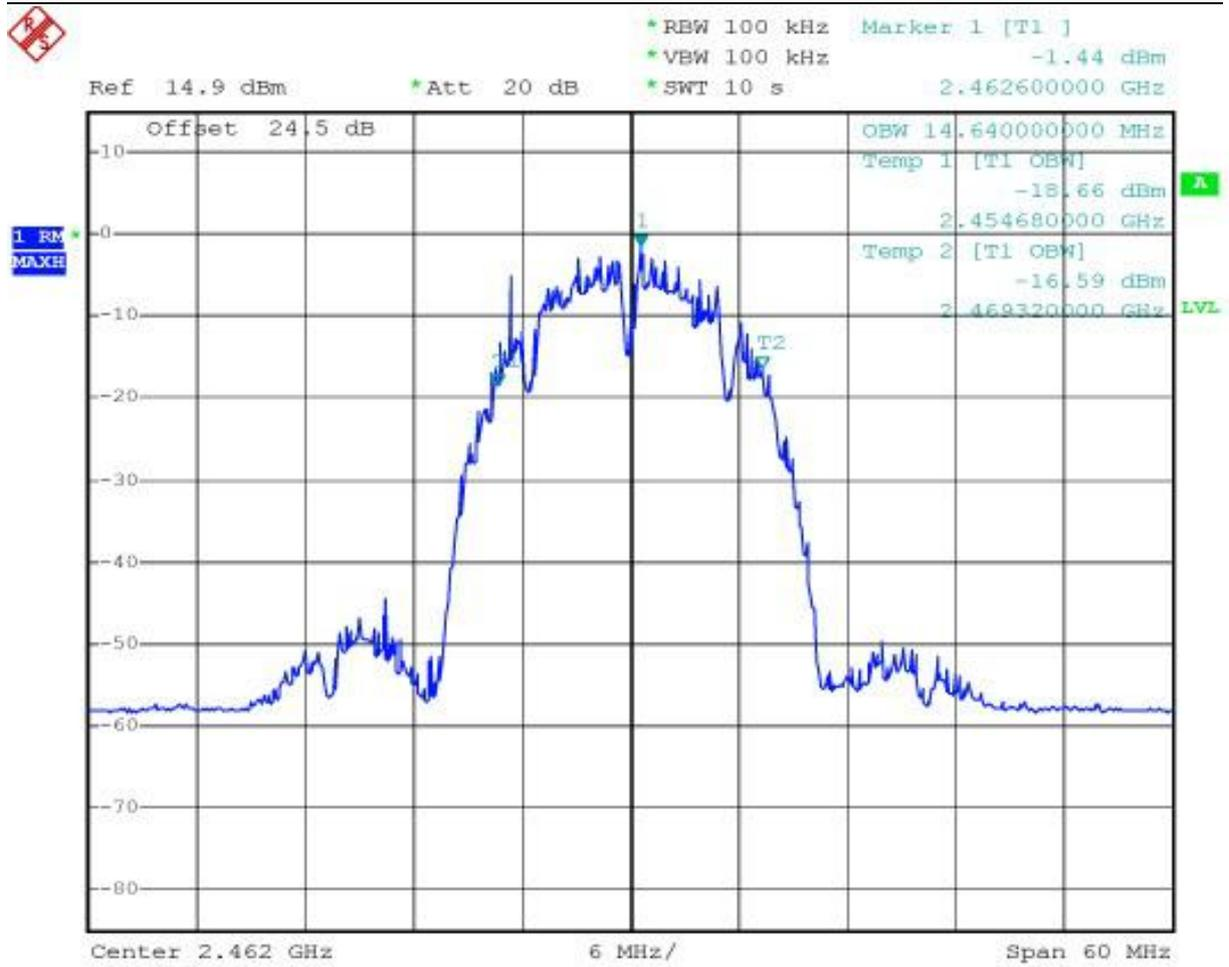
Figure 11 7104M bandwidth test curve
