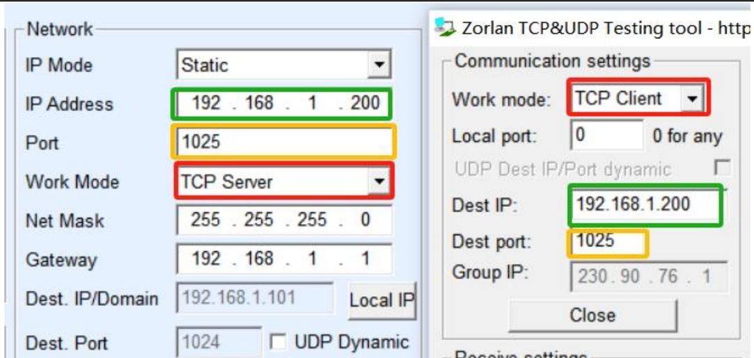
Figure 31 Serial Server as Server Side
