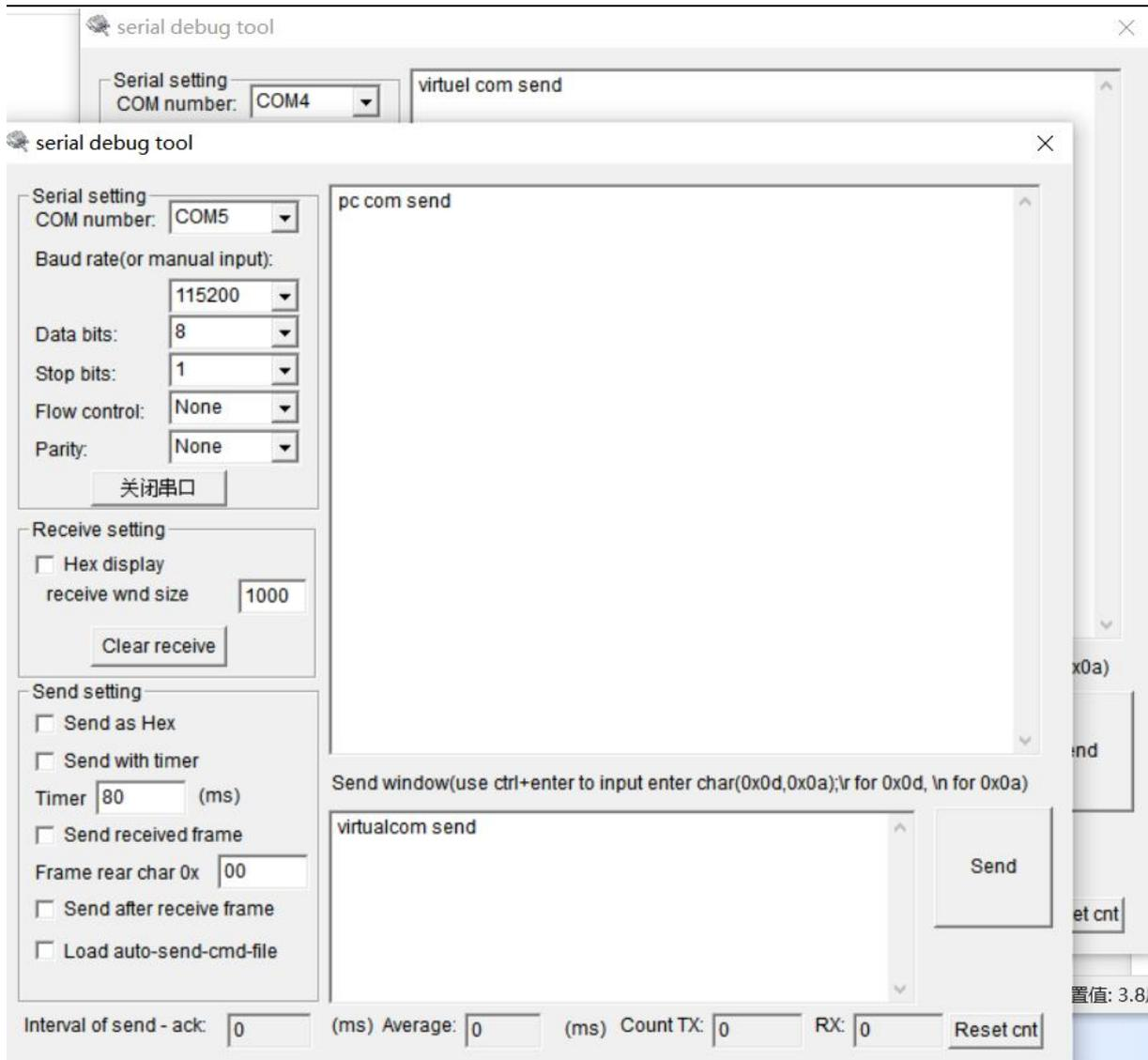
Figure 23 through virtual serial port communication
