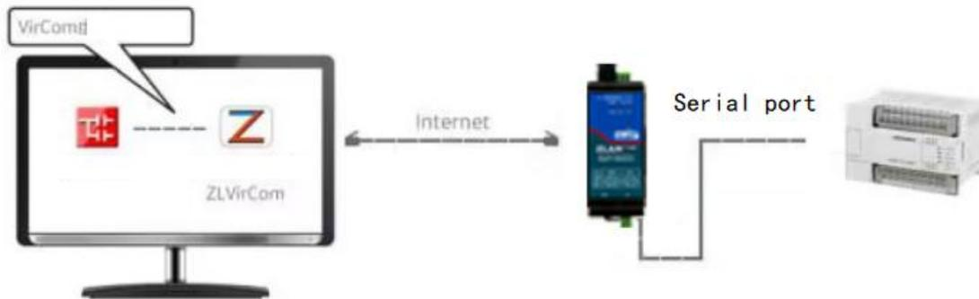
Figure 20 The role of virtual serial ports
