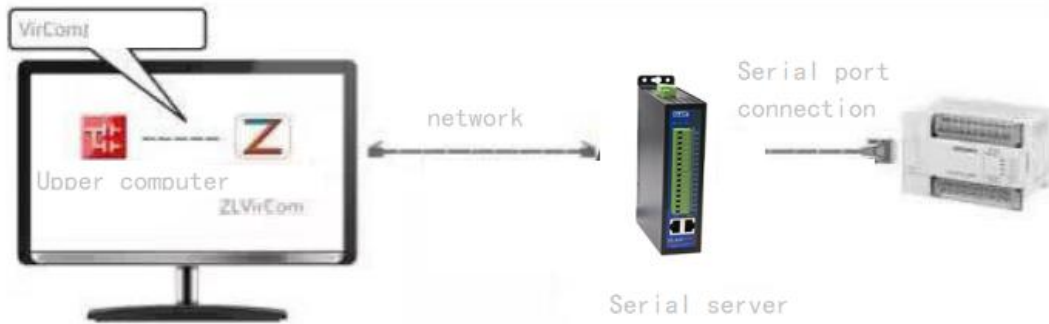
Figure 18 Functions for virtual serial port
