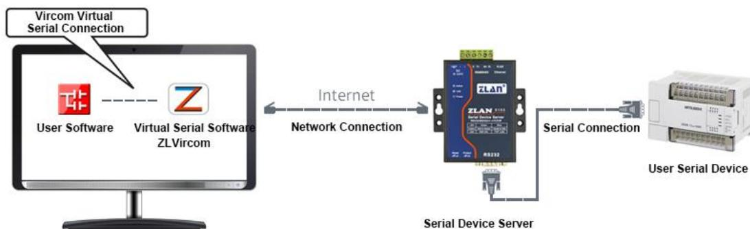
Figure 11 Virtual serial port
