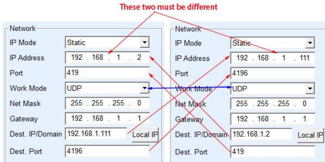
Chart 22 configuration of UDP device pairing parameters
