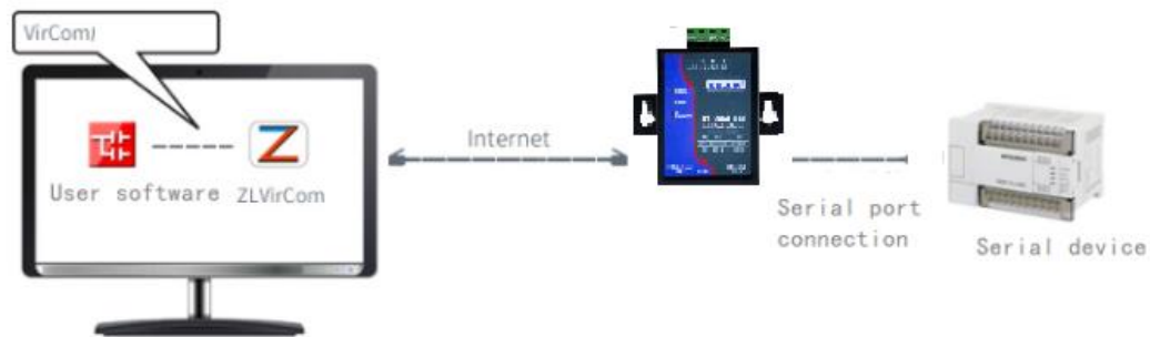
Figure 12 Functions of the virtual serial port
