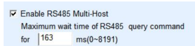
Figure 37 RS485 multi-host support
