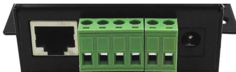
**Figure 4 Ethernet port, RS485/422 and Power Input**
