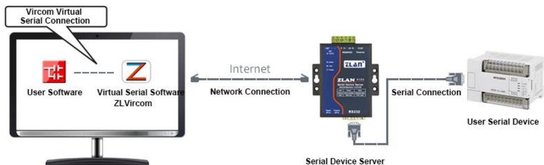
**Figure 13 Virtual serial port**
