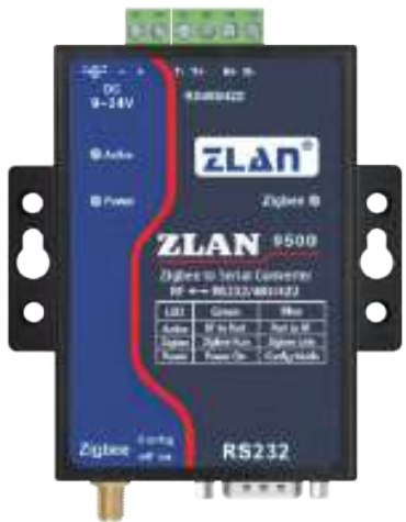
ZLAN9500 Zigbee to RS232/RS485/RS422
